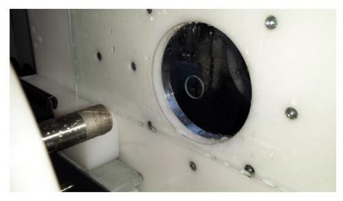
Hole in 2mm thick glass was made after 10 seconds of changing the parameters from 8mm glass drilling, which was executed before.
